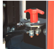
Battery Isolator Switch
